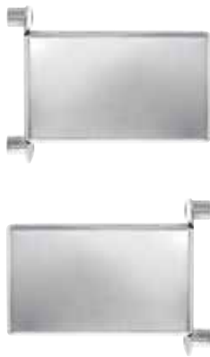
Light & CB Antenna Bracket For 2018-2022 Freightliner Cascadia • Highly polished 304 premium grade stainless steel for durability and shine • Stainless steel bracket for single stud pedestal light, and CB antenna • Mounts onto mirror arm. Simply remove two mirror arm mounting screws, install the bracket, and reinstall the longer screws included
