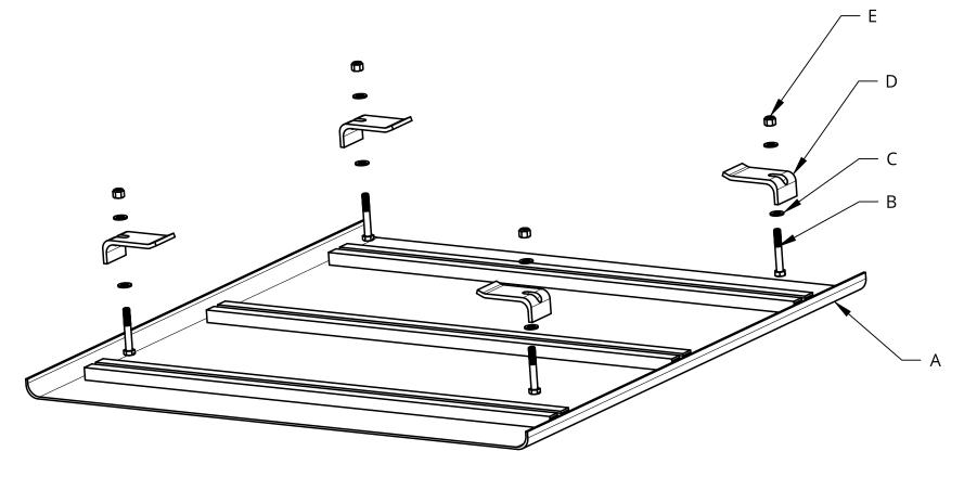
Use the "L" brackets to clamp onto truck's frame to secure deck plate.
