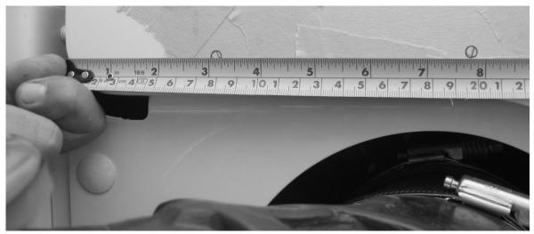
Measure and mark the horizontal placement of these holes on the previously mentioned centerline. The first hole will be located at 3-1/8" from the rear edge of the hood, while the second will be located at 7-3/4" from the rear edge of the hood.
